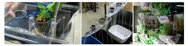
Fig. 3: (Left to Right) A sample of iterations of a hydroponic irrigation system over the course of a month from an initial vacuum formed tray configuration, to a basket configuration, to a fully secured assembly
