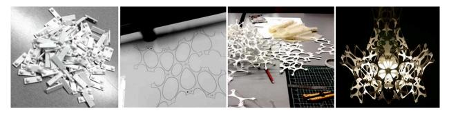
Fig. 1: (Left to Right) 3D prints of connection pieces, laser cutting of frames, assemblage of elements, and final light
